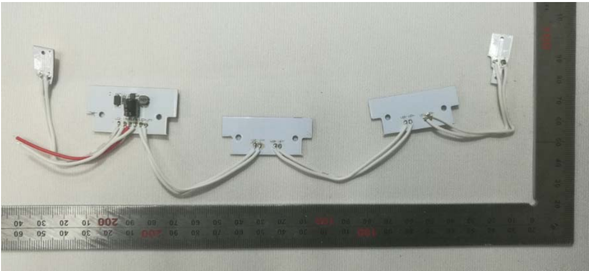
Back view of PCB for rear registration plate lamp
